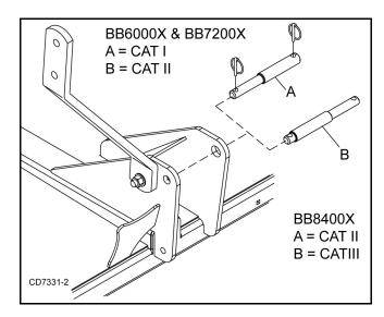
Figure 4. Mounting Pin Installation
